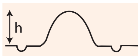
Schema del calcolo dell'indice Erichsen e del LDR (test Swift). Calculation diagram of the Erichsen index and LDR (Swift test).
