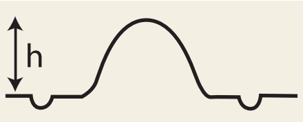
Schema del calcolo dell'indice Erichsen e del LDR (test Swift). Diagram of calculation of Erichsen index and LDR (Swift test).
